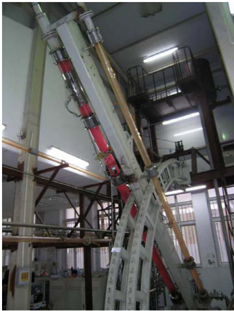
Fig. 2. Schematics of inclined oil–water two phase flow experiment.
